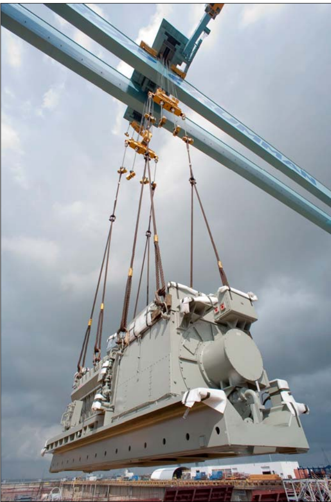
Northrop Grumman Shipbuilding lifted two generators weighing over 195,000 pounds a piece into the aft section of the nuclear-powered aircraft carrier USS Gerald R. Ford (CVN 78) on July 28, 2010. The generators supply backup power throughout the ship.
