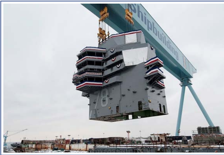
555 ton island is lowered onto the flight deck of the USS Gerald R. Ford (CVN 78).
