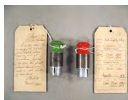
The Electronic Test Officer aboard the Enola Gay replaced three green safety plugs with three red arming plugs to activate Little Boy, the atomic bomb dropped on Hiroshima on August 6, 1945. This original safety plug is accompanied with a spare red plug taken on the mission (Courtesy of the Clay Perkins Collection).
