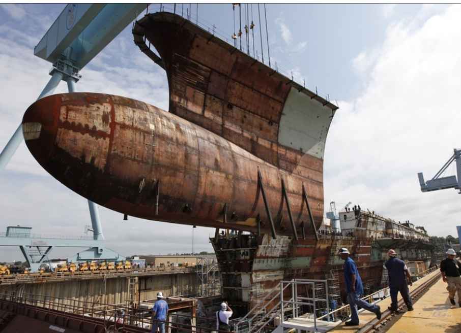
The first piece of the flight deck for the aircraft carrier Gerald R. Ford (CVN 78) was erected April 7. The 717-metric ton unit includes combat systems and electronics spaces. Photo by Chris Oxley.
