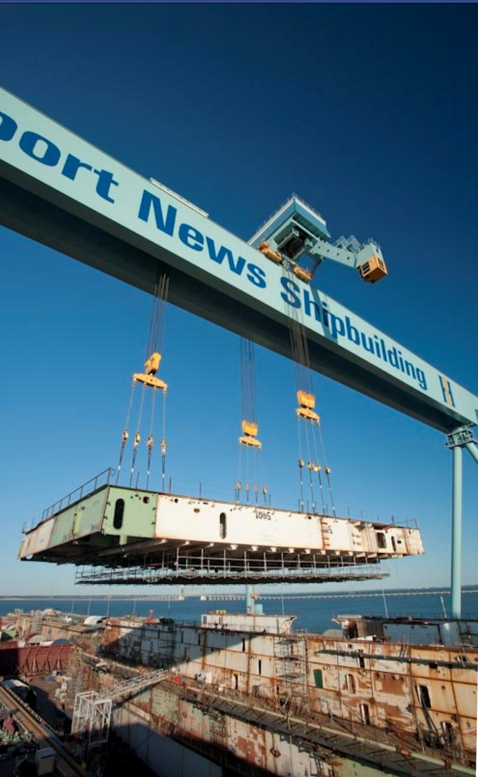
The first piece of the flight deck for the aircraft carrier Gerald R. Ford (CVN 78) was erected April 7. The 717-metric ton unit includes combat systems and electronics spaces. Photo by Chris Oxley.
